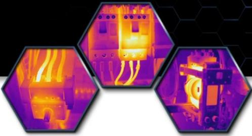
A preferred method of establishing the baseline for transmittance adjustment is to calibrate the imager using an infrared window and a target which has achieved a stable temperature in the range you anticipate your actual target to be operating in (as detailed in Madding, 20041). Doing so will give a thermographer the most accurate baseline transmissivity value. But what if that transmissivity value were to change? What effects will that change have on data accuracy?
